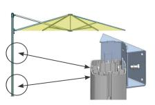
Fixing brackets are height adjustable
